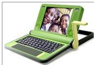
Enlarge | GETTY IMAGES This is a prototype of Design Continuum's hand-cranked $100 laptop, designed for students in developing countries.
