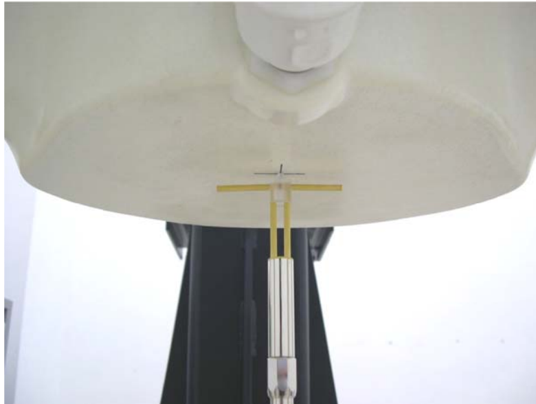
Fig 8.2 Photo of Dipole Setup
