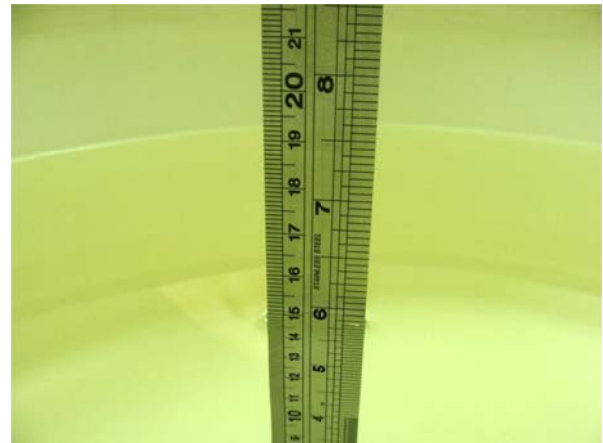
Fig 6.2 Photo of Liquid Height for Body SAR
