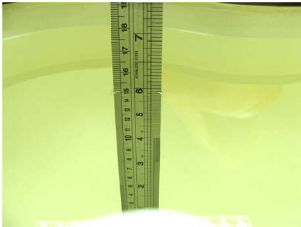
Fig 6.1 Photo of Liquid Height for Head SAR
