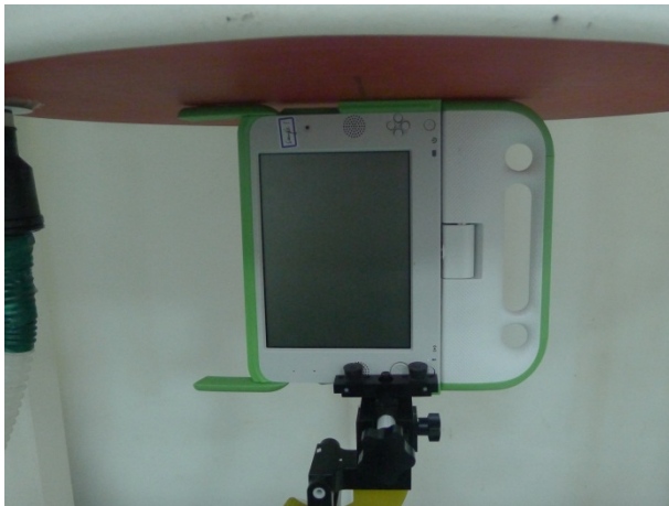
Fig 9.11 Edge2 with Phantom 0 cm – Antenna Position 180°
