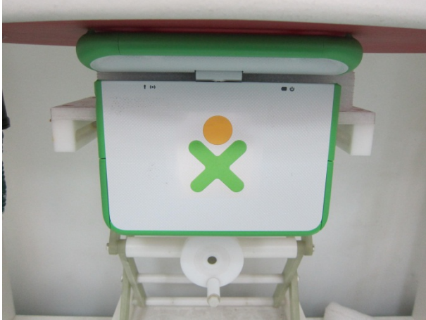
Fig 9.3 Bottom of Laptop with Phantom 0 cm Gap – Antenna Position 0°
