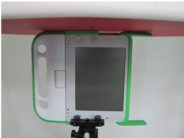
Fig 9.13 Edge4 with Phantom 0 cm – Antenna Position 180°
