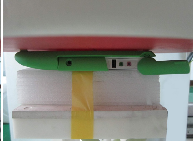
Fig 9.6 Bottom of Tablet with Phantom 0 cm – Antenna Position 180°
