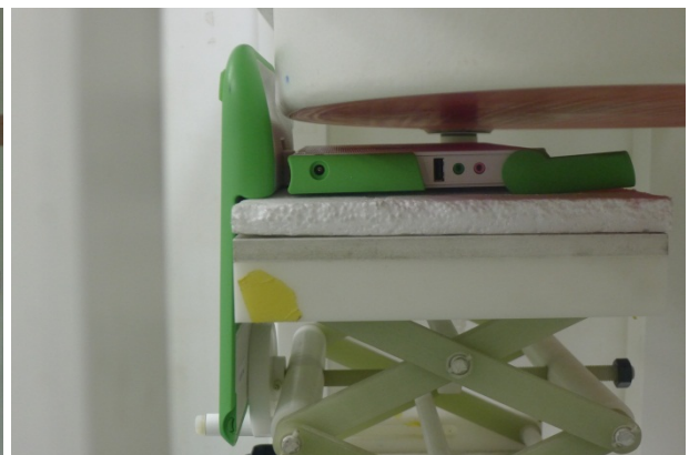
Fig 9.8 Back of Panel with Phantom 2.5 cm – Antenna Position 180°
