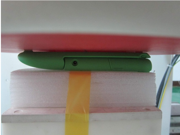
Fig 9.5 Bottom of Tablet with Phantom 0 cm – Antenna Position 0°
