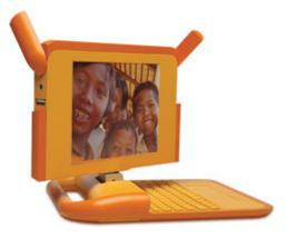
The newest prototype includes pieces that work as mesh wireless network antennae when flipped up and cover the USB and audio ports when not in use.
