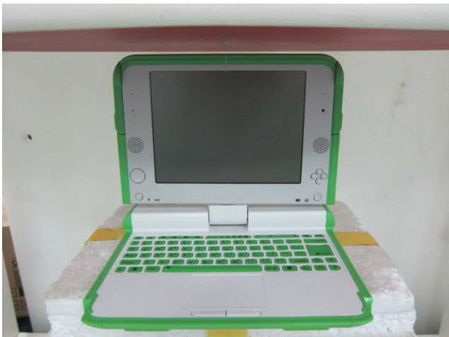
Tip of Panel in Laptop (1cm) Antenna Position 0°
