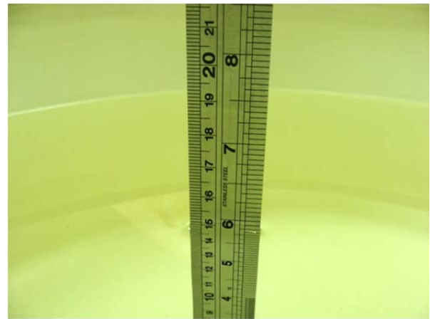
Fig 6.2 Photo of Liquid Height for Body SAR
