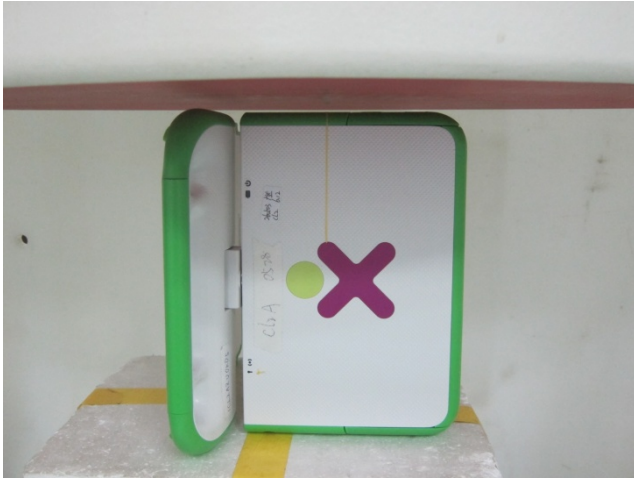
Right of Panel in Laptop (1cm) Antenna Position 0°
