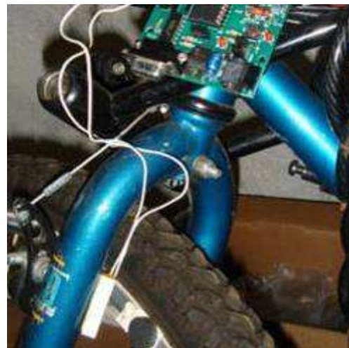
Figure 14. Magnetic sensor installed on bicycle
